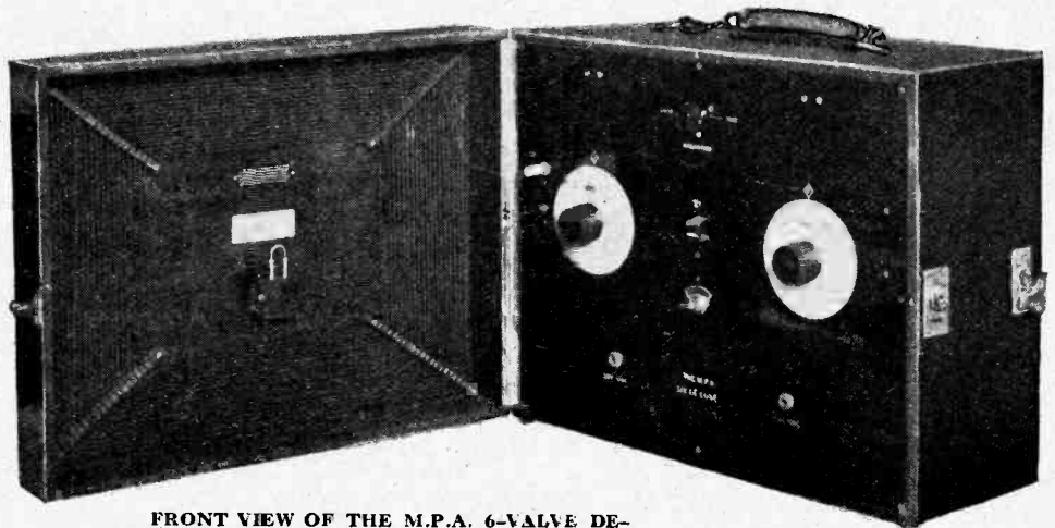
FRONT VIEW OF THE M.P.A. 6-VALVE DE-LUXE RECEIVER, showing frame aerial in lid.
